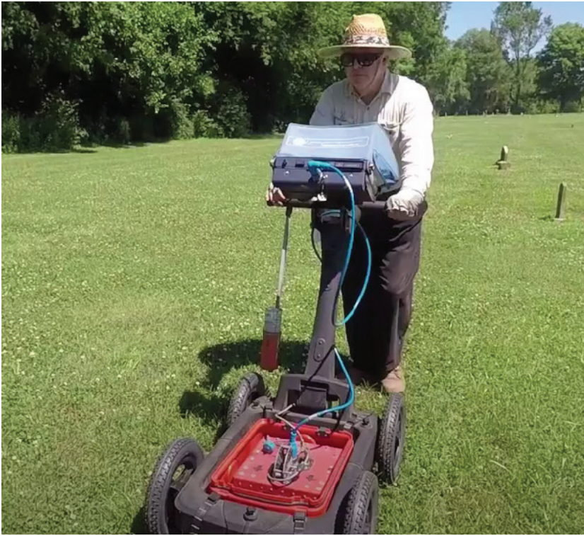
Matthew Turner conducts a ground penetrating radar (GPR) survey of the Gallatin City Cemetery.
