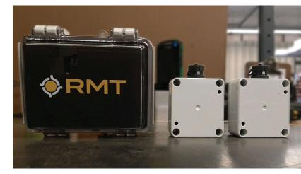
Sensors have been recently installed vehicles in the city of Gallatin's fleet that provide data on where potholes are located. The technology records vibrations and then uploads information about flaws in city streets, allowing officials to better determine the condition of each street and which streets need repairs.
