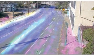
This heat map is one of the ways CUIP collects data in the testbed. Data can show different types of vehicles and pedestrians as well as places where pedestrians are crossing the street - even if there is no designated crosswalk in place.
