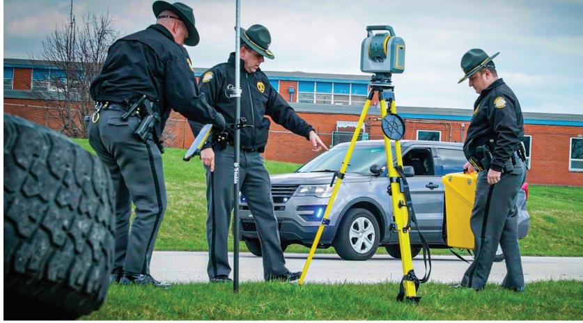
Officers use a 3D scanner to investigate a vehicle accident. The scanners can be employed on crime scenes both indoors and outdoors to collect important data for both investigations and prosecutions. By capturing the data in this way, investigators can keep a preserved copy of the crime scene and use computer technology to better calculate trajectories, distance of travel, and other factors.
